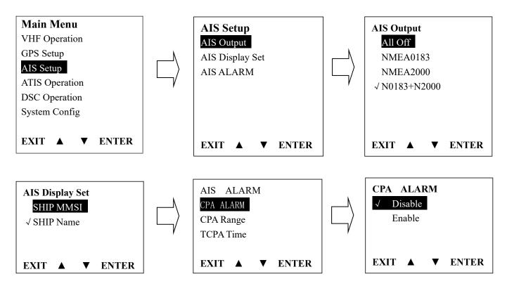
CPA Alarm enable Choose "Disable" or "Enable" item to enter disable or enable AIS alarm, then press "ENTER" key to confirm.
