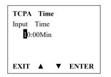
TCPA (Time closest point of approach)Alarm distance setup Press UP/DOWN key to input digital one by one, after you have done this, press "ENTER" key to confirm, the maximum input range is 30 minutes, if the input value is over than 30 minutes, the input is invalid, then the system will ask for re-enter, the default CPA value is 10:00 Min.
